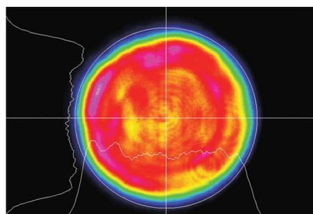
LQ215-D laser typical near field beam profile.
