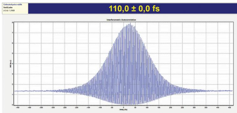
The FX150 laser typical autocorrelation curve.
