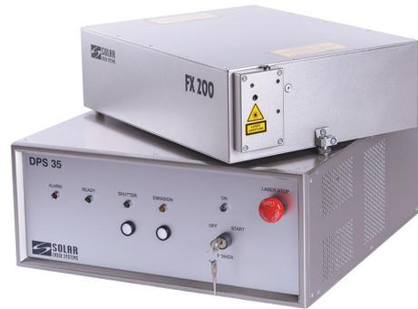
Yb-doped crystals used in these lasers allow being pumped directly by a diode eliminating the necessity in an intermediary pump laser used in traditional Ti:Sapphire lasers. For this reason the FX series lasers to the full extent combine compactness and reliability of fiber systems with advantages of solid-state technologies.
